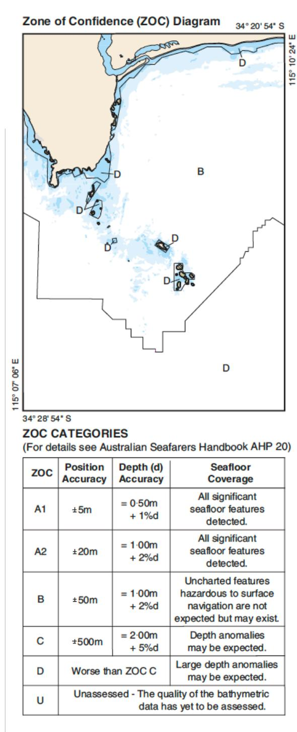
The diagram above is for the Cape Leeuwin/Flinders Bay region and is typical of south-western WA. The chart area is divided into zones (A, B, C etc.) each with a different level of accuracy. Most of the bay is zone B (position accuracy to + or – 50m), which is a lot less accurate than your GPS. The areas where the short cuts past the Cape through the reefs lie is zoned D - accuracy worse than 500m!
